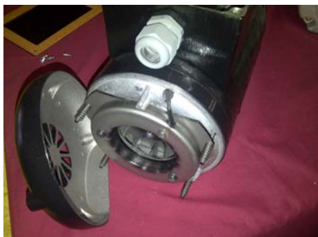
View showing fan cover removed. Note the coil housing sitting in the mounting tabs from fan baffle casting.
